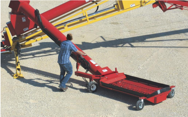
Hydraulic Drive Positions the Hopper with Ease
