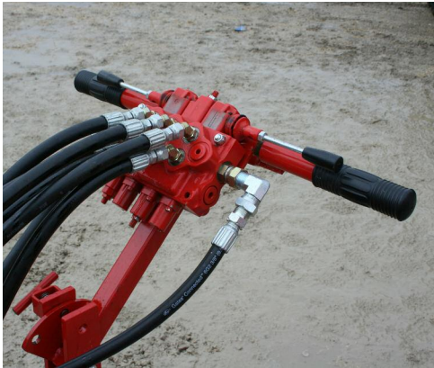
Hydraulic Handle Bar Controls
