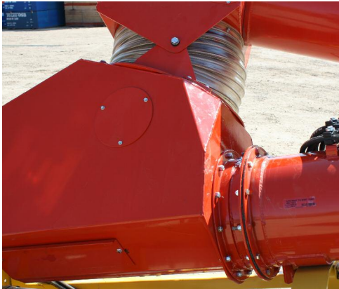
Swivel boot for efficient grain transitions and clean out
