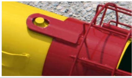
New intake "lock" to prevent the intake from shifting in transport
