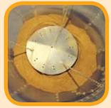
Chore-Time's SHAKER-PLATE unit causes feed to slide down the sidewall and hopper in a mass flow, continuously cleaning and polishing the inside of the feed bin. This mass flow action eliminates opportunities for feed to hang up and turn stale or moldy.
