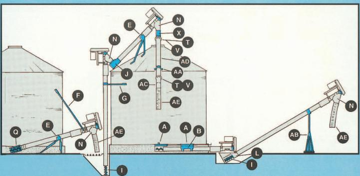
NECO's "All Purpose Auger" line consists of the same basic components used in our "Modular" line. By combining the universal power discharge head and common auger extensions with specific components, this line easily meets your customers requirements for bin unloading, bin loading, or transfer systems, regardless of bin size or system type. The customer can easily change or add on to these systems at any time without modifications.
