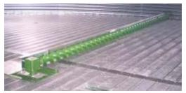
Sukup Hawk Cut<sup>™</sup> Bin Floors and Z-Post or Super Supports provide a solid base for your grain. Sukup Hawk Cut<sup>™</sup> floors are extra-strong since no steel is removed while creating the open areas in the planks.
