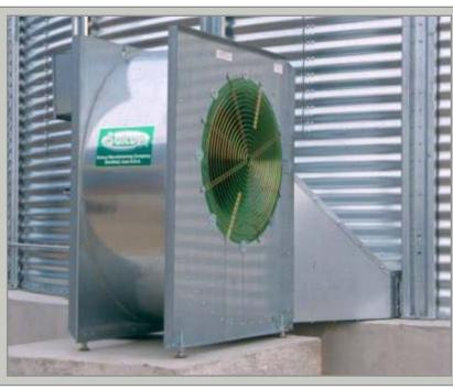
• Exclusive lip easily connects the fan to the heater or transition to form an air-tight seal.
