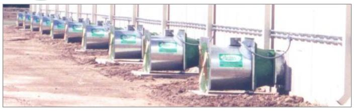
Sukup In-Line Centrifugal Fans are ideal for almost any high static pressure application, such as aerating or drying small grains, aerating tall bins, or cooling grains in roof dryer bins. In-Line Fans provide excellent airflow beyond the range of a standard axial, without the noise of an axial fan.
