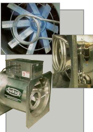
Approximate Temperature Rise: high-temp models: 50° - 180°F low-temp models: 25° - 75°F super-low temp models: 10° - 30°F  Stainless Steel Flame Sensor is more reliable and will last longer than flame probes.
